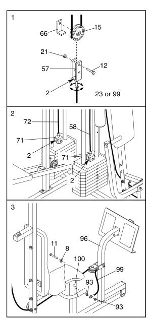
Do not overtighten the cables; the top weight will be lifted off the weight stack.
